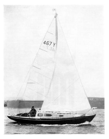
(Above) the simple masthead sloop rig is easy to handle and the boom is set high enough to clear the cockpit by a generous margin. Areas are: mainsail 170.8 sq. ft.; genoa 255.2 sq. ft.; working jib 158.2 sq. ft.; spinnaker 570 sq. ft. (Below) This shot from aft gives a good idea of the roomy and well protected cockpit and the easy access to the accommodation.
